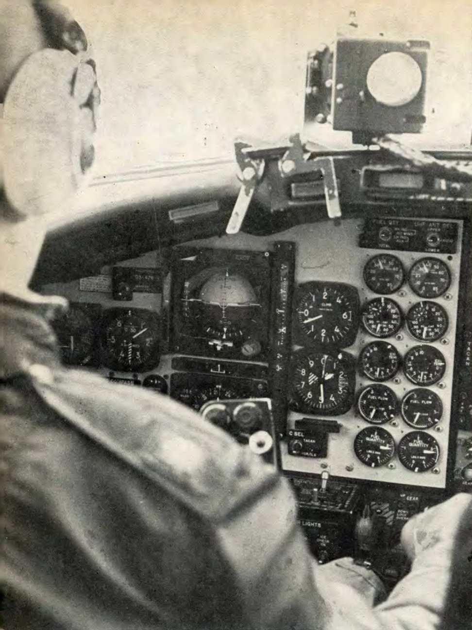
Instrument panel on specially equipped T-39 contains special instruments described in article. Note vertical indicators on each side of attitude director indicator. Photo below shows movie camera and radar altimeter mounted on glare shield.
